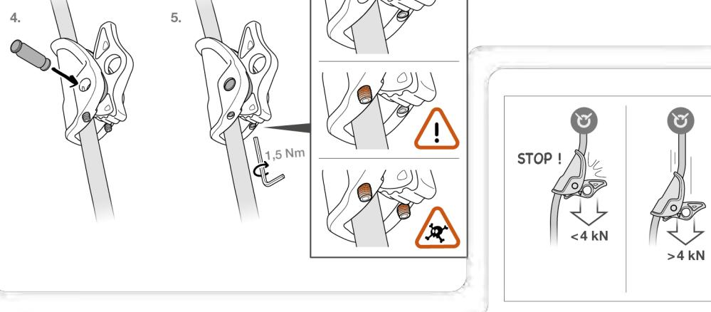
**6. Function principle and test
