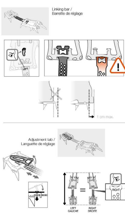
**C. Rear binding system adjustment /**
