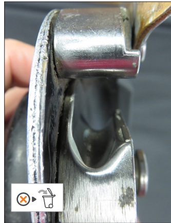
• Cam groove worn to wear indicator
