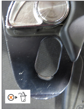
• Attachment hole deformed by a shock load
