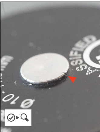
• Rivet slightly cracked
