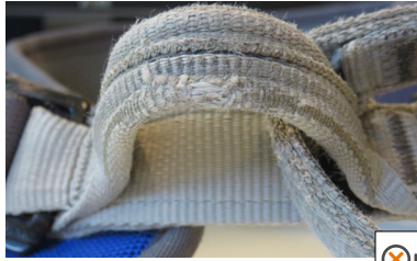
• Worn tie-in point
