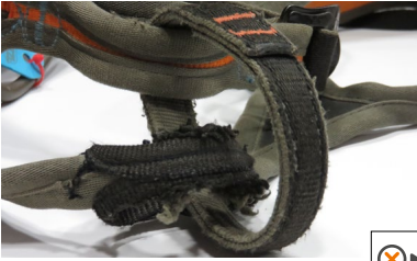
• Worn tie-in point
